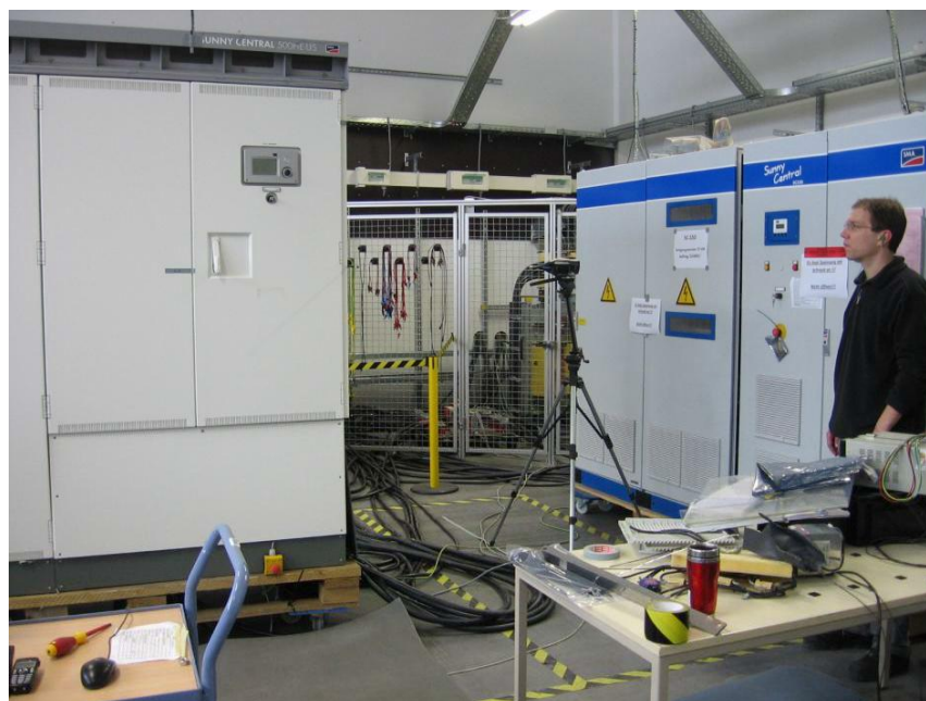
Test setup for sound level measurement with FFT determination of the frequency range and the amplitudes from the right in accordance with EN 3744
