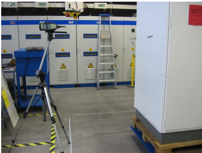
Test setup for sound level measurement with FFT determination of the frequency range and the amplitudes from the left in accordance with EN 3744-3-2
