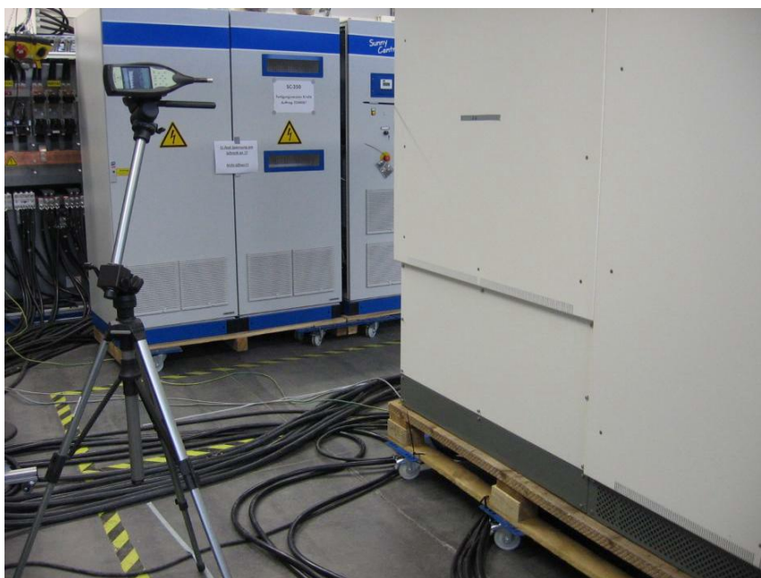
Test setup for sound level measurement with FFT determination of the frequency range and the amplitudes from the backside in accordance with EN 3744-3-2
