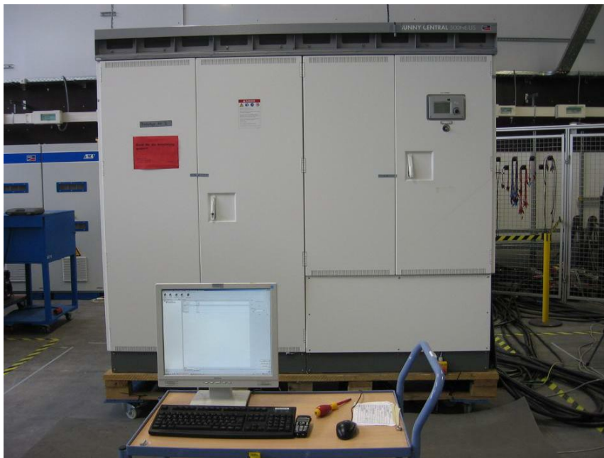
Test setup for sound level measurement with FFT determination of the frequency range and the amplitudes frontally in accordance with EN 3744
